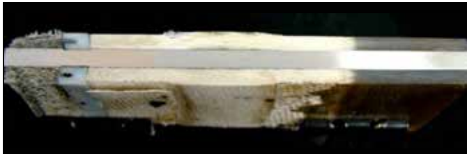
Steam attack on GRE isolation gasket
