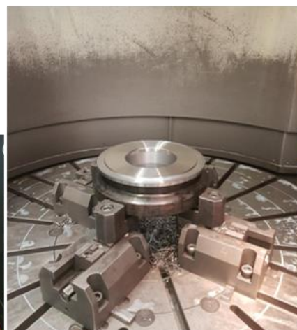
Machining after Inconel overlay
